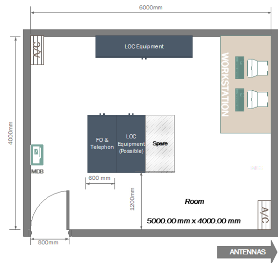
Figure 5: Typical Localiser Shelter Layout
